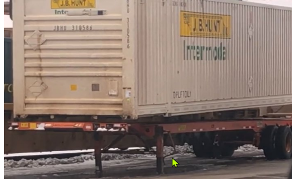
1. Container angled down on chassis
