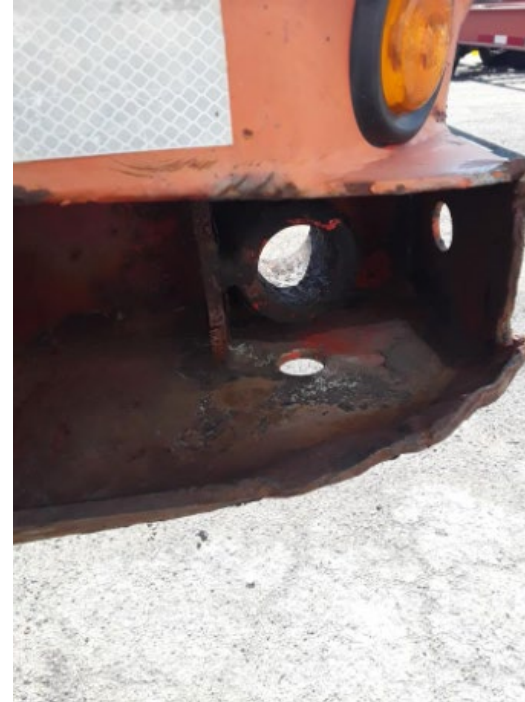
Broken/missing pin and housing
