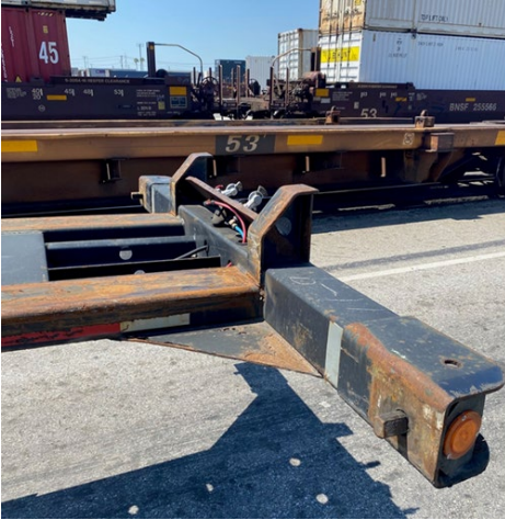
Chassis trackside with front pins engaged
