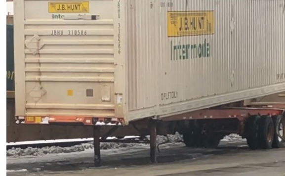
2. Container forced down and slid until impact with front bolster *
